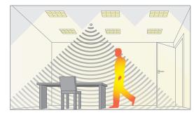
PIR movement sensors work by detecting the movement of body heat. Ideal for spaces where a defined detection pattern is required.
