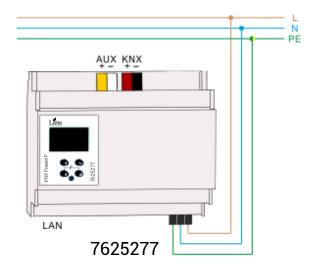
The Lime KNX PowerIP combines the central functions of a KNX bus line in a compact device (GTE): a 640 mA bus power supply with inductor, IP router and IP interface. In addition to the bus voltage, the power supply also has an auxiliary voltage output. The IP router in the device allows the forwarding oftelegrams between different lines via a LAN (IP) as a fast backbone. Via the interface function the KNX line can be addressed directly from a PC.
